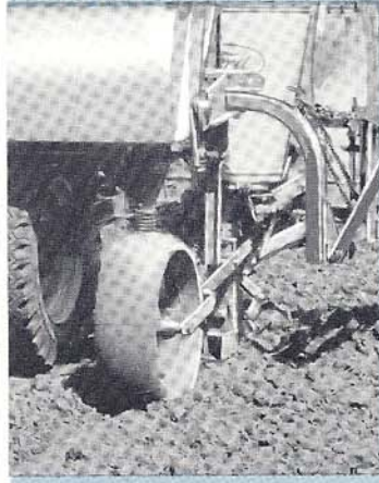
Rubber-tired Press Wheels. For firming soil and gauging depth, the steel press wheels are available with rubber tires.
